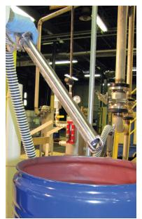
The stainless steel wand is equipped with a stand-off that prevents suction against the sides of the bulk container and helps to break up clumps of solid material.
