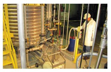
The dye container rests on a scale alongside the mixer, and the mix proportions are monitored closely to guarantee the accuracy of the final solution.
