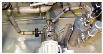
The inline SLIM Solid/Liquid Injection Manifold instantly disperses powders in a liquid stream. A specially designed rotor/stator generator develops an intense vacuum, which draws the powder through the powder injection inlet to the high shear zone, where it is dispersed instantly. An auxiliary pump and eductor are not required.
