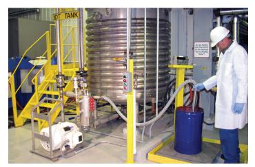
In this application of SLIM powder injection technology, a wand is used to minimize "dusting." The powder is drawn from within the bulk container, through the wand and flexible tube to the mixer, where it is injected into the liquid stream and dispersed instantly. It then recirculates through this 1,000-gal vessel until discharge.
