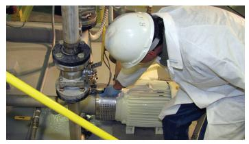
After the mixer has been started, the powder injection valve is opened. A powerful vacuum then begins to draw powder directly into the high shear mix chamber.
